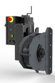
The GSM motorized compact bar hoist is designed to be a self-contained hoist with onboard controls that can be either wall mounted or mounted to the header steels of an existing or new installation.
